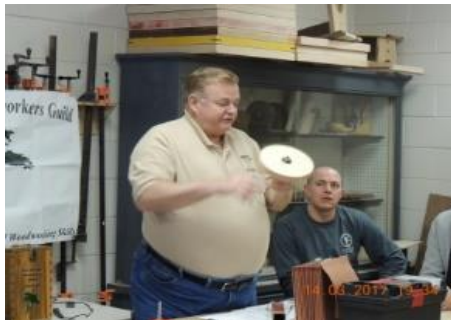
Garry Strout explaining his shop-built Honing Strop Wheel he can mount on his Lathe or in his Drill Press for honing tools in his shop.
