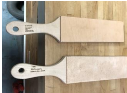
Two-sided Honing Strops The top side has smooth Leather The bottom side has rough Leather
