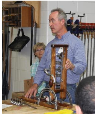
Guild Board Member, John Pflug, describing an antique Timber Framing mortising jig he restored and how it is used. He noted that when used properly it could rival the speed of today's power equipment. (Patti Dooley in the Background)
