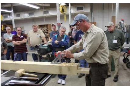
John Pflug using a Right Angle Drill and Framers Square to hollow-out a Mortise.
