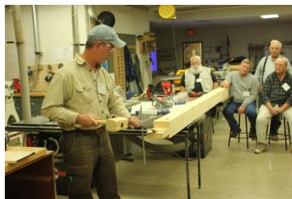
John Pflug using a 2" chisel to knock off the sawed blocks from the tenon cheeks of the tenon he is creating.
