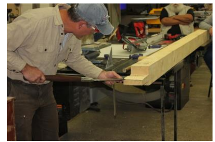
John Pflug using a 2 1/2" 'Slick' chisel to finish sizing the cheek of the tenon.
