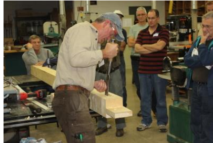
John Pflug using a 2" chisel to square-up and clean-up the inside walls of the rough mortise.
