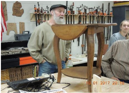
Doug Scott's "Show & Tell" Table project. A round solid walnut table with three drop leaves and tapered and curvilinear legs.
