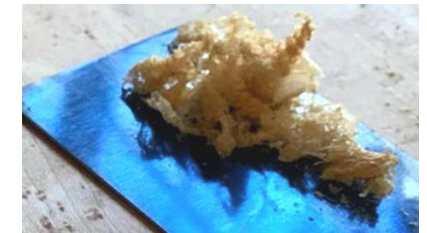
When a card scraper is sharpened correctly, the above is the result you should get when scraping a wood surface. Fine wood shavings that remove the 'Bumps, Lumps and Unevenness' of a finely and/or highly figured or straight grained wood surface that you cannot remove or level with just hand sanding.
