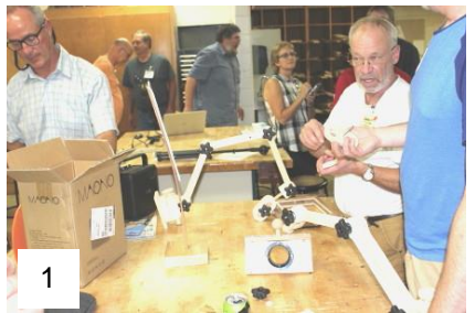
Pic. #1, the sliding router jig for flattening wood slab, table tops or work bench tops. Pic. #2. Darin Tuttle explains the set-up of the router with either a standard flat bottom router bit or the use of the 3” carbide tipped router bit. Pic. #3, Darin talking about how to lock down the slab so it cannot move while flattening it and how to deal with twists in an un-flattened natural slab. Pic. #4, Darin flattening the 14” wide, 8’ long walnut slab donated by Guild member, John Pflug.
