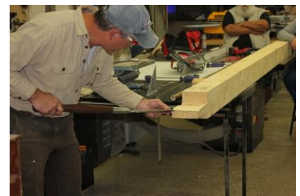
John Pflug using a 2 1/2" 'Slick' chisel to finish sizing the cheek of the tenon.
