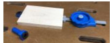
The clamp is an In-Line style made of plastic; a simple knob drives the clamp, screw style. It applies up to 250 lbs. of force and holds very well. The impressive part is how easy they are to apply and release.
