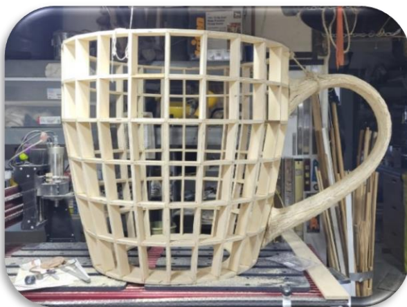
Handle from 7 layers of marine plywood
